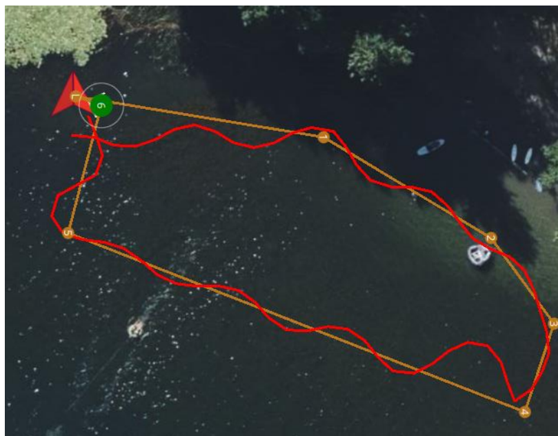
Figure 26: Current tuning after additional PID tuning.
