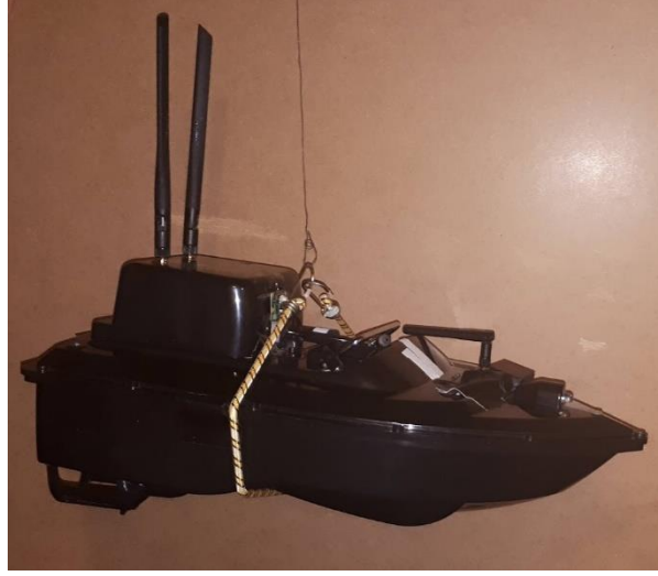
Figure 9: Autonomous boat suspended from torsional spring
