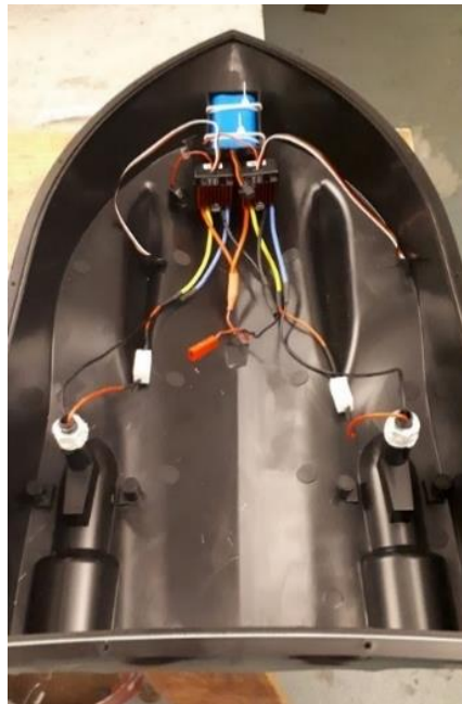
Figure 3: USV hull with upgraded motor controllers and battery.
